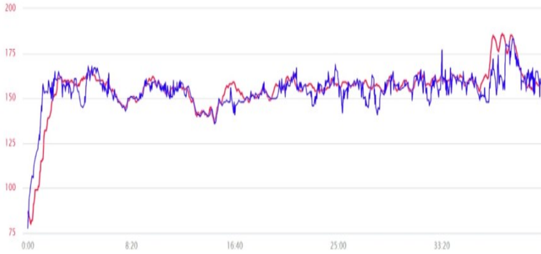
FIGURE 2.2: Comparison of heart rate measurements between a Garmin heart rate chestbelt (red) and the Cosinuss o One sensor (blue), following [44].
